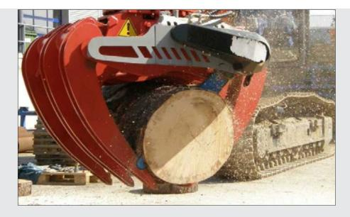
The customer's requirement was to develop a special grapple, which should be able to cut concrete piers.
