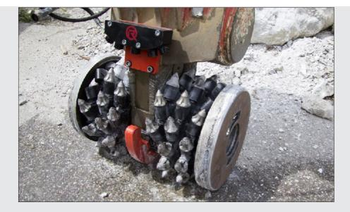
The customer's specification was a hydraulic cutter, wich could mill a small profiling depth (3mm).
